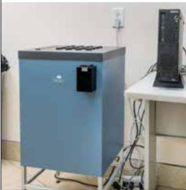
The Isothermal Calorimeter is an excellent tool to determine cement hydration kinetics and monitor the cement hydration process. The hydration profiles from calorimetric tests can predict sulfate balance, strength development potential and cement compatibility in concrete mixtures as well as helping to troubleshoot concrete performance issues in the field.
