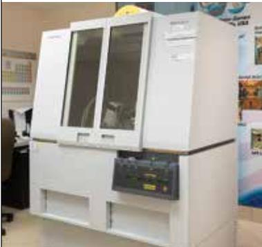
The QXRD is an excellent tool to evaluate the mineral phases in materials. It reveals important features of cement minerals including the "true" amount of individual phases, the type of calcium sulfate, and polymorphism of calcium silicates, aluminates and ferrite. The information provides guidance to the cement processing condition. More importantly, it is a powerful tool for troubleshooting performance issues in the field.
