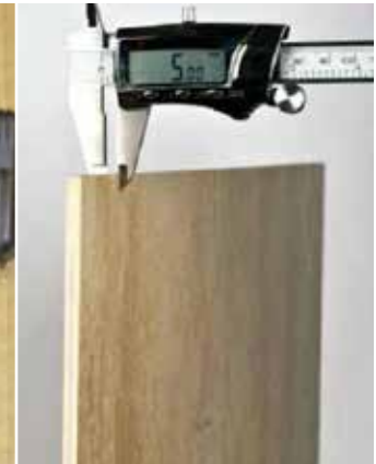
Example of a gauged porcelain tile panel/slab 5 mm thick
