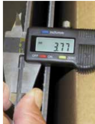
Example of a gauged porcelain tile panel/slab 3.5 mm (3,5 mm) thick with reinforcing mesh
