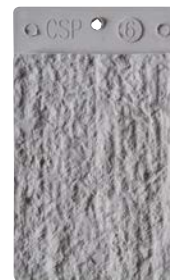
ICRI CSP 6: Medium scarification
