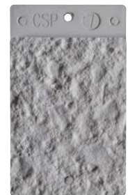
ICRI CSP 7: Heavy abrasion blast
