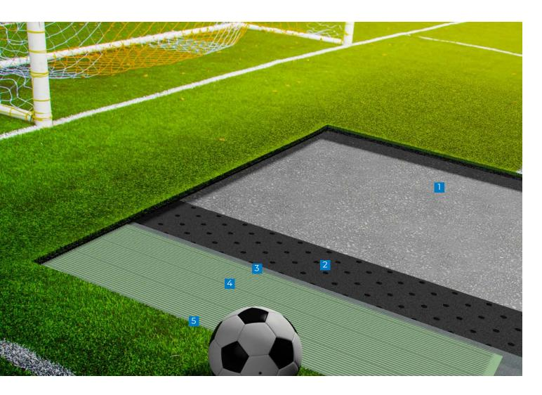
When it comes to the incredible stresses on a synthetic-turf football field during training and games, it is critical to ensure that the sub-base and seam strength are up to the task. *Mapesoil* products offer a great solution to create a strong sub-base that will last for the lifetime of the field.
