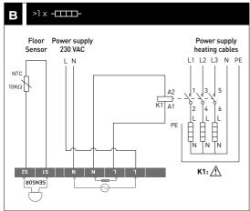
$lack \Delta$  Do not use contactor without suppression device.
