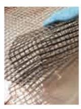
Rete 320 Glass fibre mesh for reinforcing epoxy systems.
