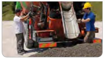
After mixing for a few minutes with **RE-CON** ZERØ, concrete is transformed into granular material which may be discharged on the ground and, once cured, used as aggregate in concrete. **RE-CON** ZERØ works with all types of concrete.
