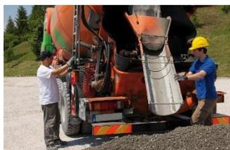
Image 3 – Aggregates formed from returned concrete using Re-Con Zero Evo
