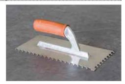
To spread the adhesive on the back of the tiles, on the other hand, use a spreader with smaller notches (square notches of at least 3-4 mm) so that almost 100% of the surface is wetted with adhesive.
