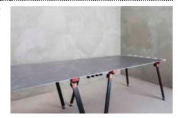
When making a straight cut, place the cutting guide on the tile along the line to be cut and block it in place with suction cups.
