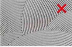
The adhesive must be spread in the same direction on the back of the tile and on the substrate (in straight lines parallel to the short side of the tile).
