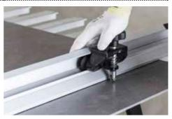
Then complete the cut from one end to the other, making sure you apply the same amount of pressure on the cutting tool for the entire length of the cut.
