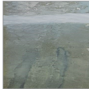
Mapecoat I 600 W diluted 1:1 with water
