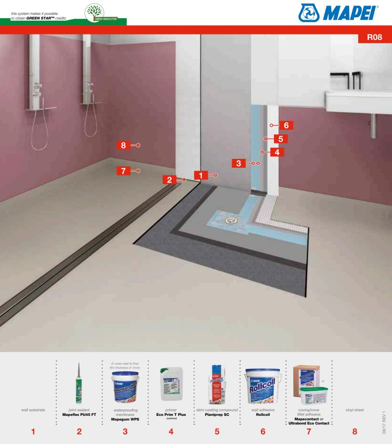
Resilient System – Internal Installation of Vinyl Sheet on Walls in Wet Areas
