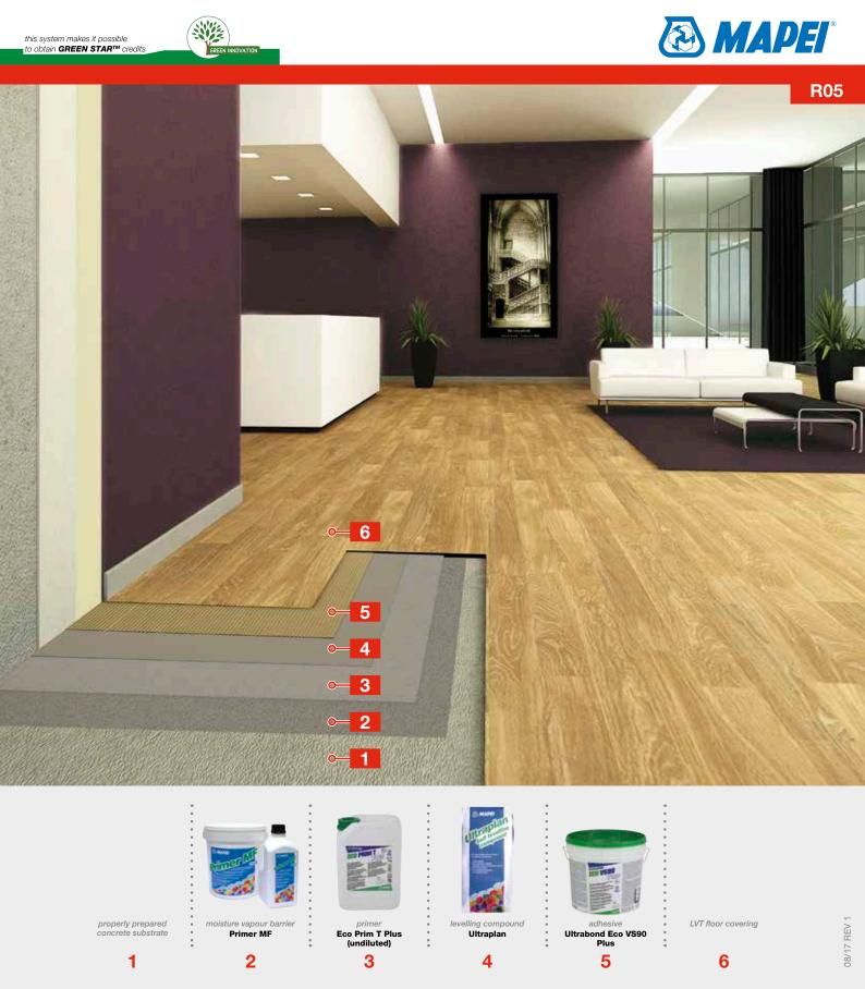
Resilient System – Internal Installation of LVT over Concrete with High Residual Moisture
