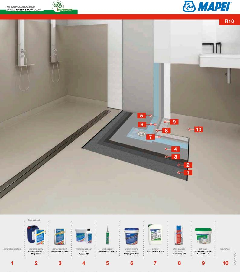
Resilient System – Internal Installation of Vinyl Sheet on Floors in Wet Areas
