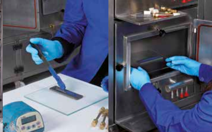
Test to measure VOC emissions
