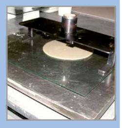
MAPEI's Research and Development laboratories are also at the forefront in the research into self-levelling and thixotropic smoothing compounds, using the most innovative testing and analytical methods. In particular, the application of new experimental techniques allows MAPEI to optimise the characteristics of their own self-levelling compounds according to requirements, which are dimensionally stable, with high self-levelling capacities, high mechanical strength and excellent workability.
