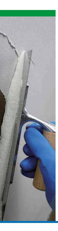
**Planitop Smooth & Repair R4:** Structural R4-class, rapid-setting, shrinkage-compensated, thixotropic, fibre-reinforced, cementitious mortar, applied in a single layer between 3 and 40 mm thick, for repairing and smoothing concrete.
