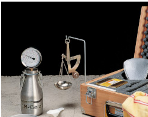
Carbide hygrometer for measuring the moisture level of a Mapecem screed
