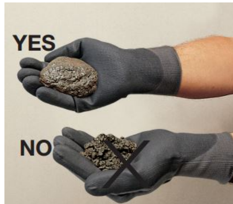
The correct consistency of Mapecem
