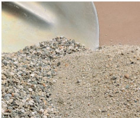
Aggregates for Mapecem: gravel from 4 to 8 mm and sand from 0 to 4 mm
