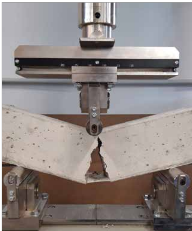
Picture taken in the laboratory showing the crack-bridging capacity of Mapeproof FBT .
