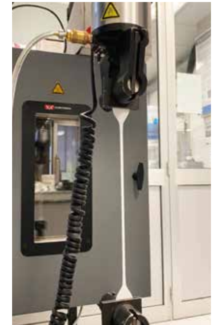
Mapei laboratory: extension test on the membrane.
