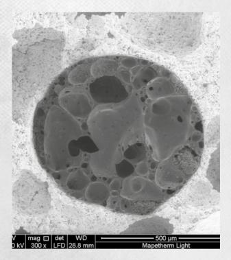
An image through an electron microscope showing a section of the honeycomb air pocket structure in the lightweight aggregate, which helps give Mapetherm AR1 Light its lightweight characteristics.
