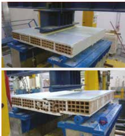
Anti-tipping protection for buffer and dividing walls subjected to orthogonal flexure. Increase in deformation capacity of up to 500% without losing any load-bearing capacity.
