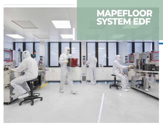
Self-levelling epoxy system with a high solids content for antistatic, dissipative industrial floors, thickness 1.5 to 2 mm.
