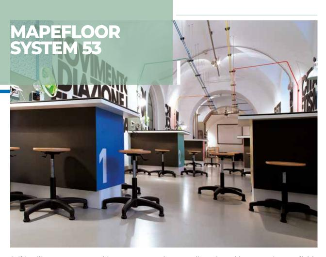
Self-levelling vapour-permeable epoxy system in water dispersion with a smooth matt finish; thickness up to 4 mm.
