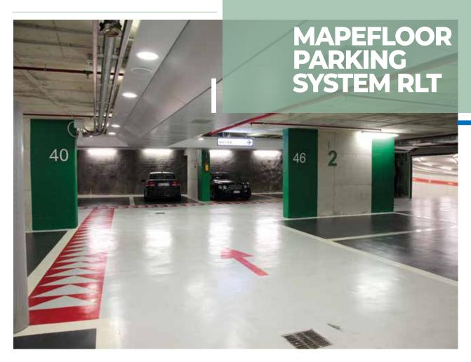
Multi-layered, seamless epoxy system for pedestrian surfaces and areas with vehicle access exposed to light traffic. The system complies with the Guidelines of the German Committee on Reinforced Concrete OS 8 and the concrete surface protection systems according to EN 1504-2; thickness 0.8 to 1.2 mm.
