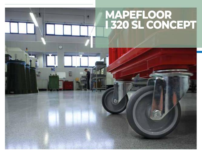
Self-levelling epoxy system with a coloured granular finish for decorative floors; thickness of approx. 2 mm.
