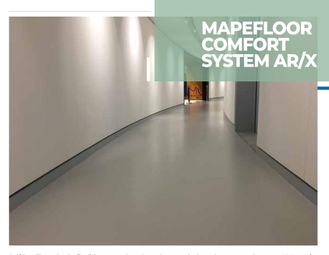
Self-levelling, elastic, flexible, aromatic polyurethane resin-based system resistant to UV rays for coating surfaces in internal surroundings; thickness 6 mm.
