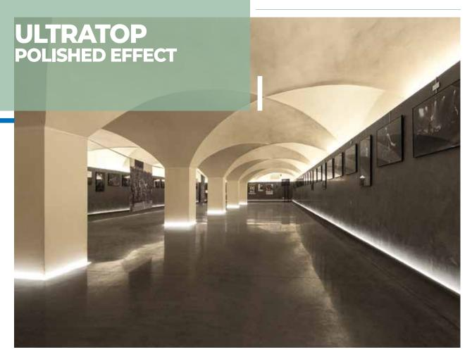
Self-levelling, ultra-fast setting cementitious system for abrasion-resistant floors with a polished effect; thickness 10 to 40 mm.
