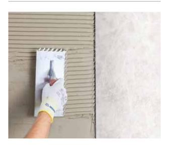
One-component, rapid-setting and -hydration, high-performance, highly deformable, lightweight, cementitious adhesive with extended open time, and extremely high yield. It is easy to apply by trowel and features excellent back-buttering capacities, Low Dust technology, and very low emission of volatile organic compounds. It is classified as C2FES2 according to the standards EN 12004 and ISO 13007-1, as well as EMICODE EC1 Plus by the GEV.
