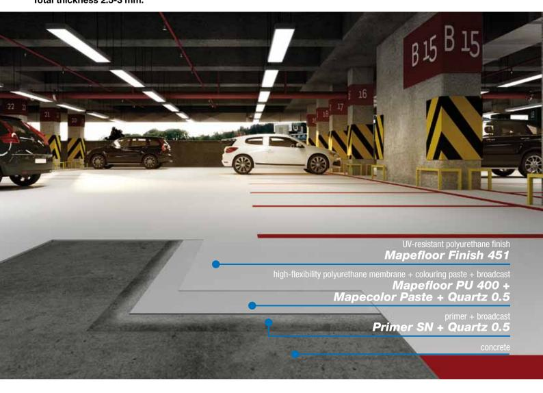
Flexible, non-slip, multi-layered, coloured coating system with crack-bridging capacity at temperatures down to -20°C. Suitable for creating strong, impermeable and waterproofing\* coatings with high chemical resistance on internal surfaces, including those subjected to variations in temperature, such as:
