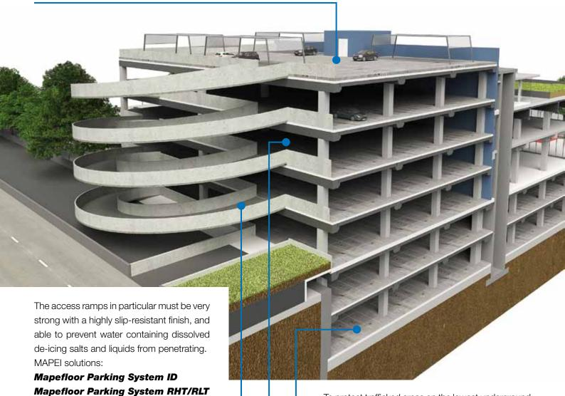
The intermediate floors must offer protection against mechanical wear and aggressive chemicals, and also prevent de-icing salts from penetrating into them, but the movements due to expansion and contraction of the substrate are less compared with the top floor. MAPEI solutions:
