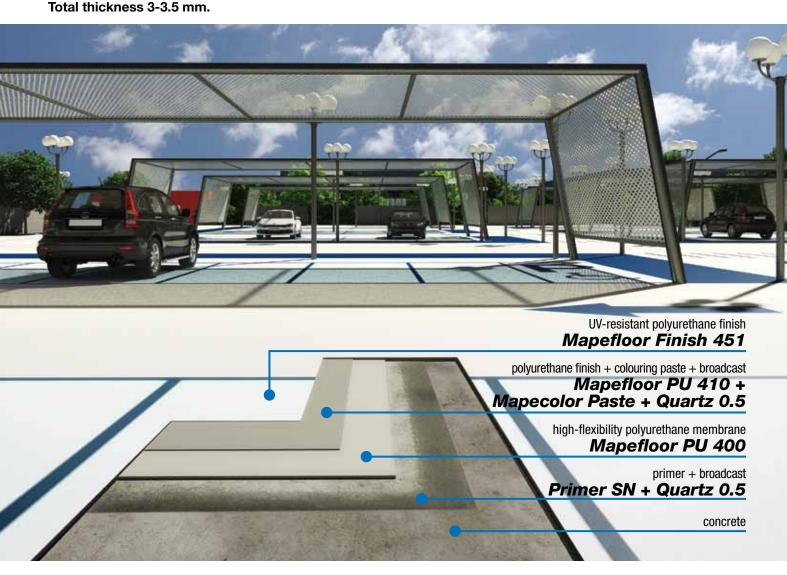
Highly elastic, slip-resistant, multi-layered, coloured coating system with *crack-bridging* capacity down to -20°C. Suitable for creating strong, waterproofing\* coatings with high chemical resistance on both internal and external surfaces in:
