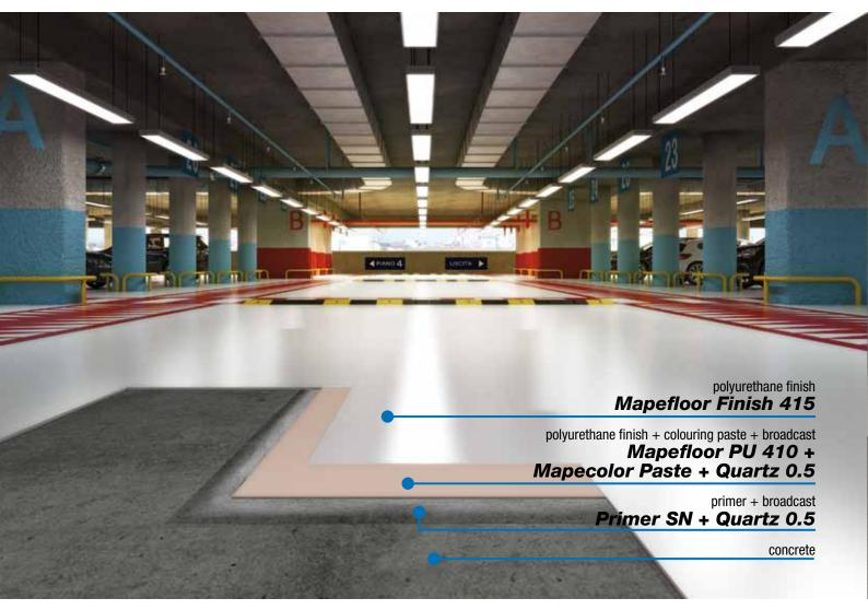
Flexible, non-slip, multi-layered, coloured coating system. Suitable for creating strong, waterproofing\* coatings with high chemical resistance on internal surfaces, including those subjected to moderate variations in temperature:
