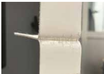
Mapei laboratory: peel test on SealLap.
