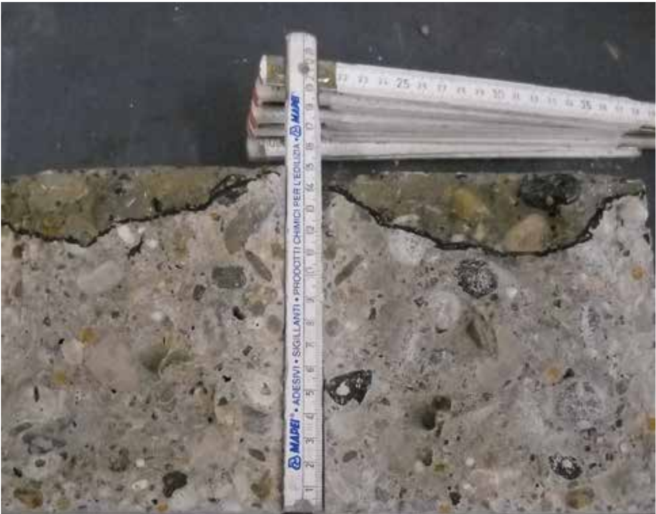
Effect of Idrocrete KR 1000 on the maximum penetration depth of water in concrete
