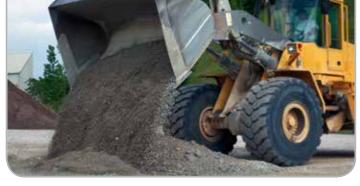
After mixing for a few minutes with **RE-CON** ZERØ or **RE-CON** ZERØ **EVO**, concrete is transformed into granular material which may be discharged on the ground and, once cured, used as aggregate in concrete. **RE-CON** ZERØ or **RE-CON** ZERØ **EVO** work with all types of concrete.
