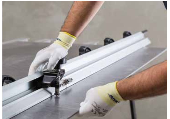
Making a cut in a tile
