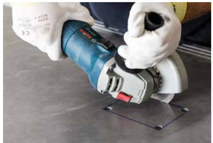
Sequence to make a rectangular hole
