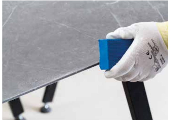
Smoothing off the cut edges
