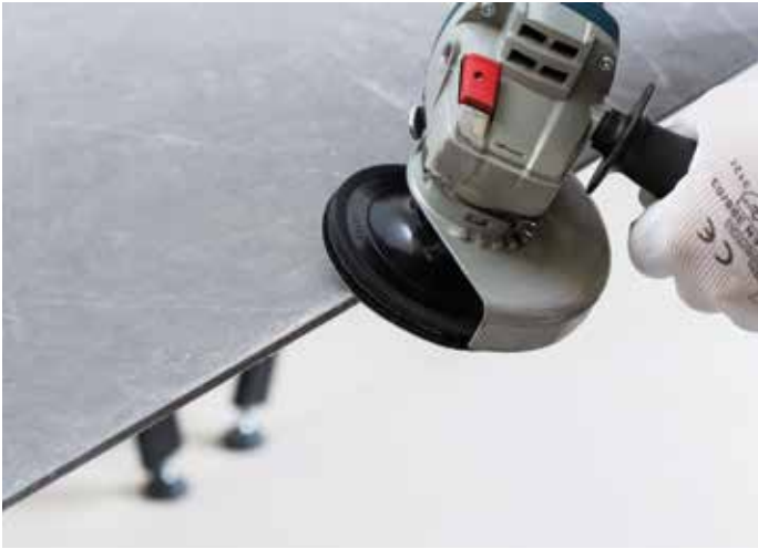
Smoothing off the cut edges
