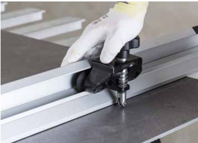
Making a cut in a tile
