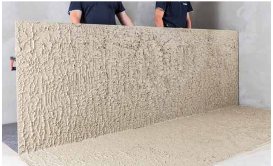
Choosing adhesive with good wetting capacity on the back of the tile
