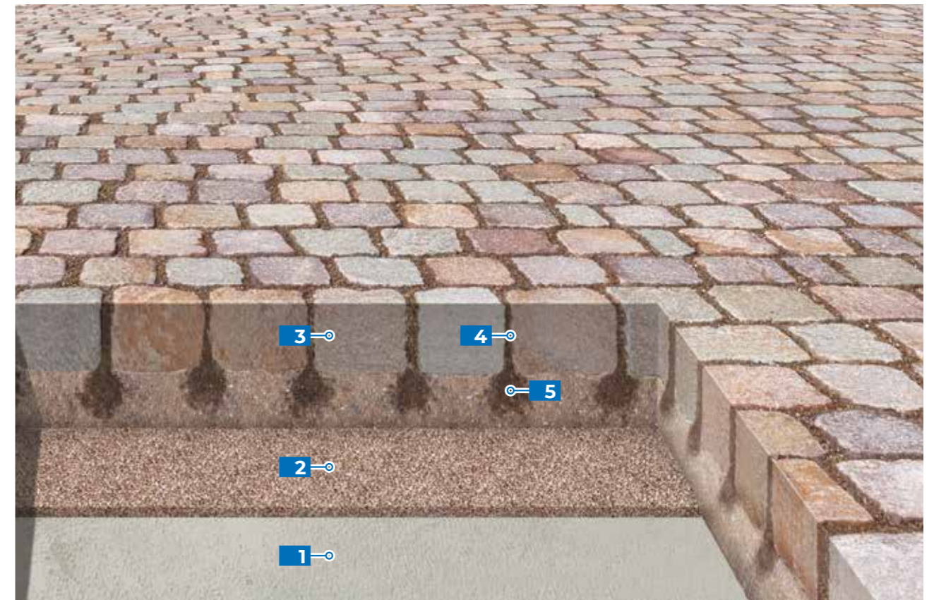
TYPICAL SECTION OF SETTS PAVING GROUTED WITH MAPESTONE JOINT, MAPESTONE JOINT GHOST OR MAPESTONE JOINT GHOST PLUS
