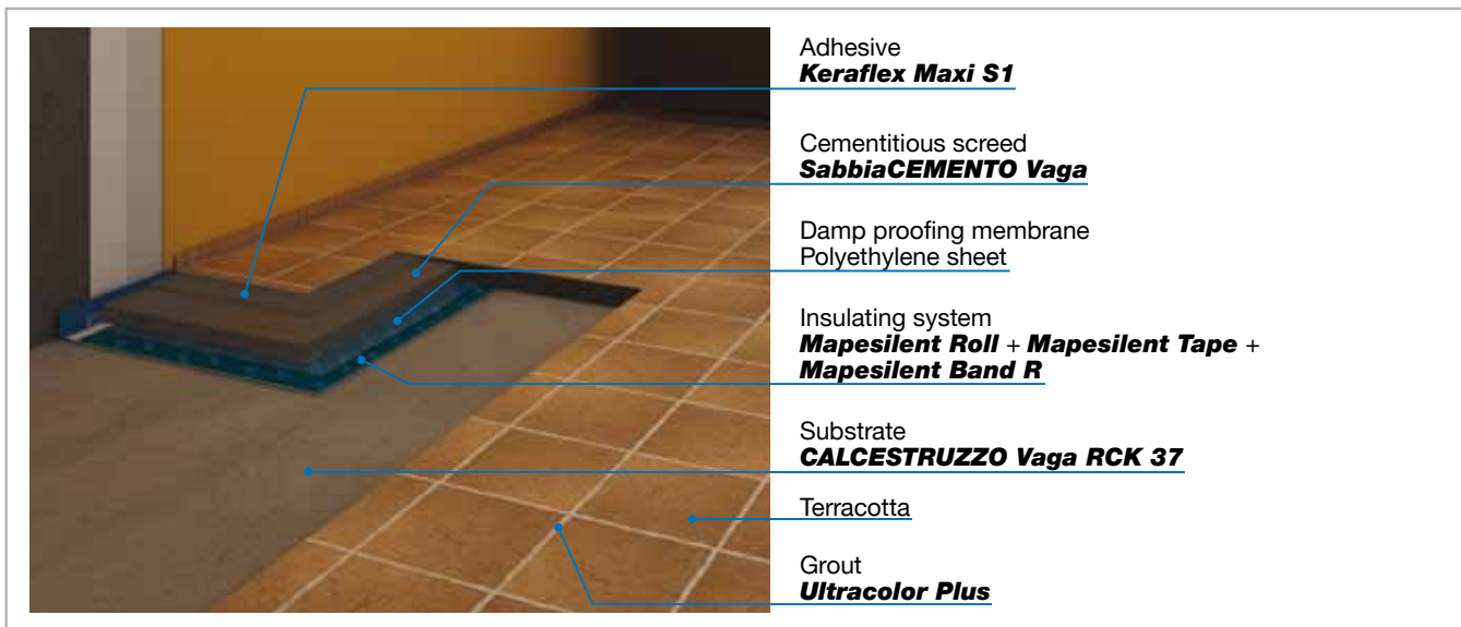
Fig. 4.3.2 - Floating screed soundproofed with MAPESILENT SYSTEM
