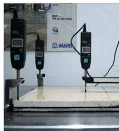
Fig. 2.3 - Dimensional stability test by bonding with quick-hardening adhesive
