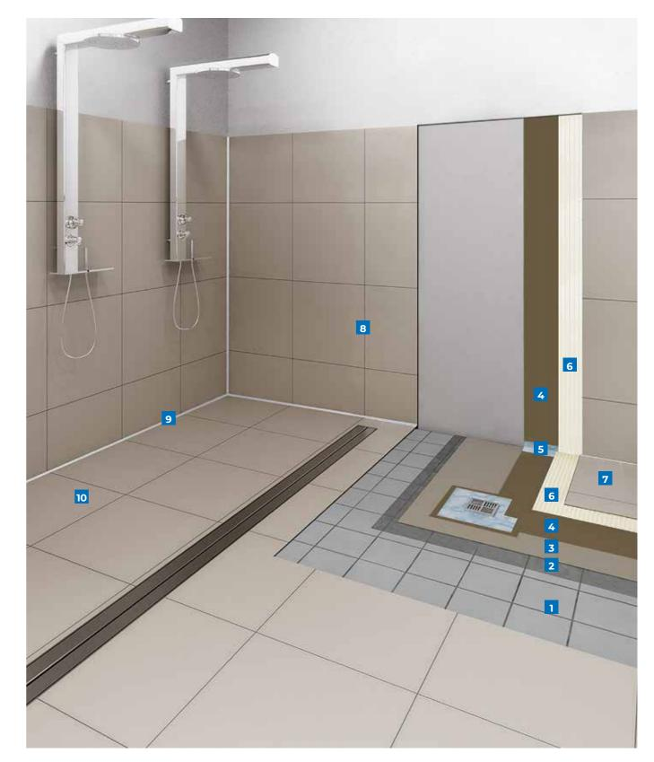
1 Old flooring 2 Eco Prim T Plus 3 Planex HR Maxi 4 Mapelastic Turbo 5 Mapeband Easy
