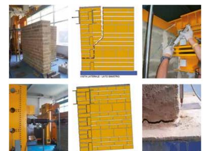
"T" intersection to dissipate more energy than the test piece without strengthening, and without any significant modification to its initial rigidity, and prevent the collapse mechanism that had been observed in the test piece without strengthening.
