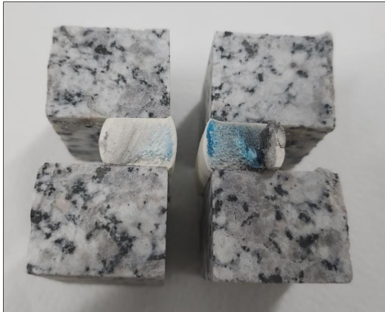
Upper substrate: with primer Lower substrate: without primer
