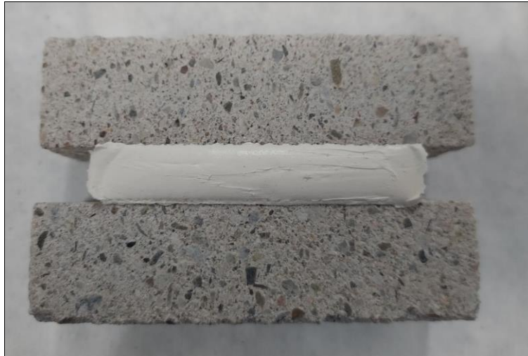
Upper substrate: with primer Lower substrate: without primer
