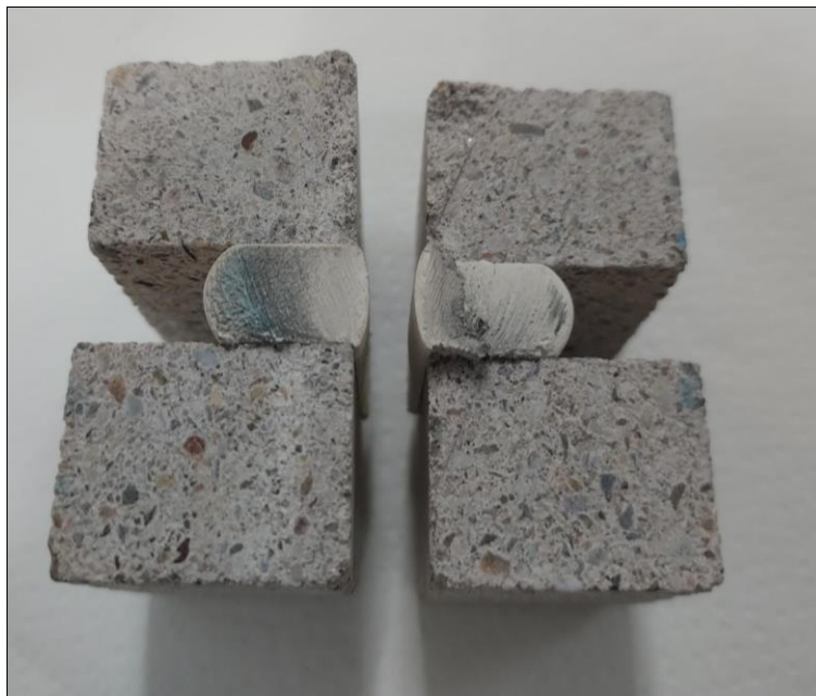
Upper substrate: with primer Lower substrate: without primer
