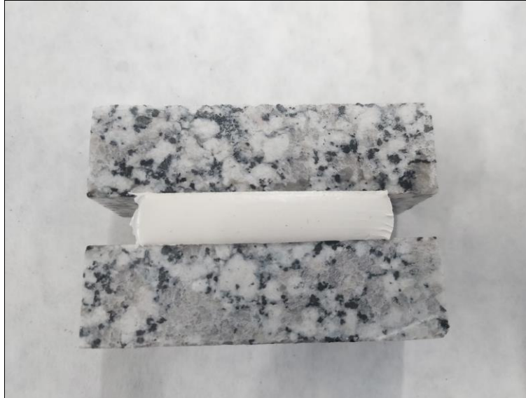
Upper substrate: with primer Lower substrate: without primer
