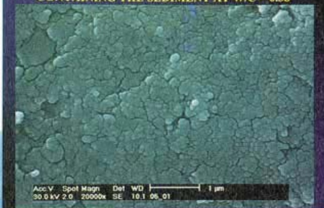
FIG. 10 SEM IMAGE OF FRACTURE AREA OF MORTAR CONTAINING THE SEDIMENT AT W/C = 0.38
