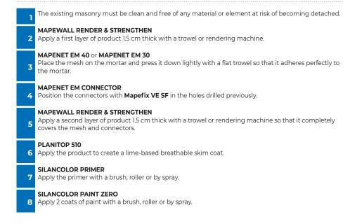
CEMENT-FREE PURE HYDRAULIC LIME-BASED SKIMMING AND RENDERING SYSTEM FOR LEVELLING OFF AND RESTORING MASONRY, INCLUDING MASONRY WITH OLD PAINTWORK
