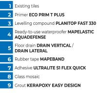
SYSTEM FOR INSTALLING LVT/SPC IN DAMP ENVIRONMENTS INCLUDING OVER EXISITNG CERAMIC TILES
