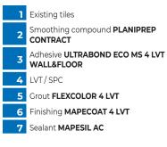
SYSTEM FOR INSTALLING DECORATIVE WALL COVERINGS AND LVT/SPC IN DAMP ENVIRONMENTS INCLUDING OVER EXISITNG CERAMIC TILES
