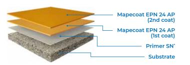
\*For anti-slip, broadcast Quartz sand (final system thickness will be 1 – 1.5 mm).
