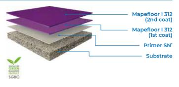
\*For anti-slip, broadcast Quartz sand (final system thickness will be 1 – 1.5 mm).
