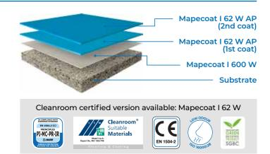
Environments: Electrical rooms - switch rooms and transformer rooms, Areas with light vehicle and foot traffic, Damp areas such as car-washes, agricultural and industrial warehouses, etc., Cementitious surfaces in cleanrooms.
