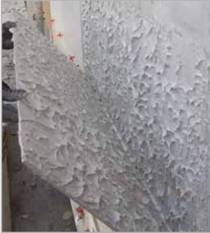
Fig. 4.13 - Wetting capacity of adhesive with Ultralite technology
