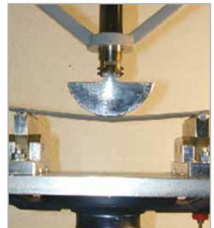
Fig. 4.7 - EN 12004 flexure test for adhesives
