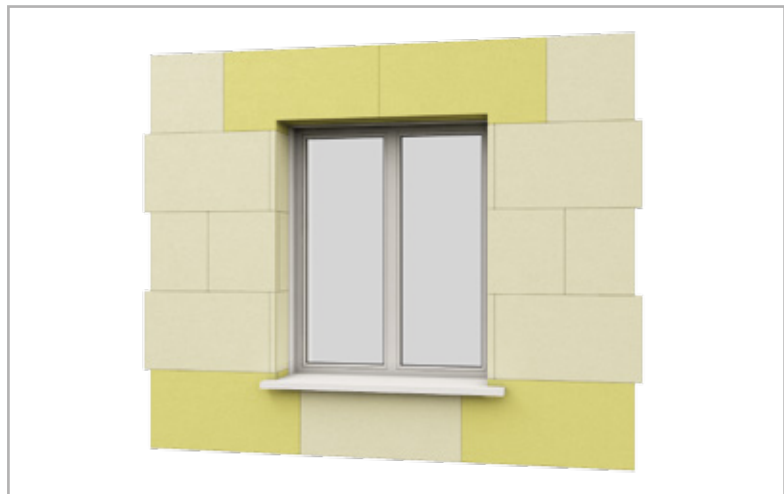
The correct way to position panels around openings
