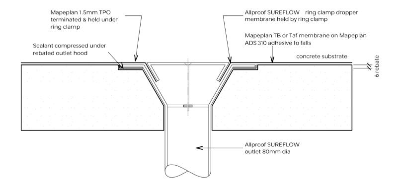
Generic drawing only. Used as a guide for design. Project specific drawings must be created for construction
