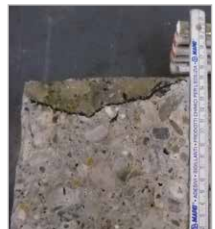
Fig. 9.3 - Concrete with a water/cement ratio of 0.45
