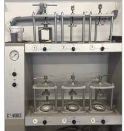
Fig. 5.1 - Equipment used to carry out a water penetration test on concrete
