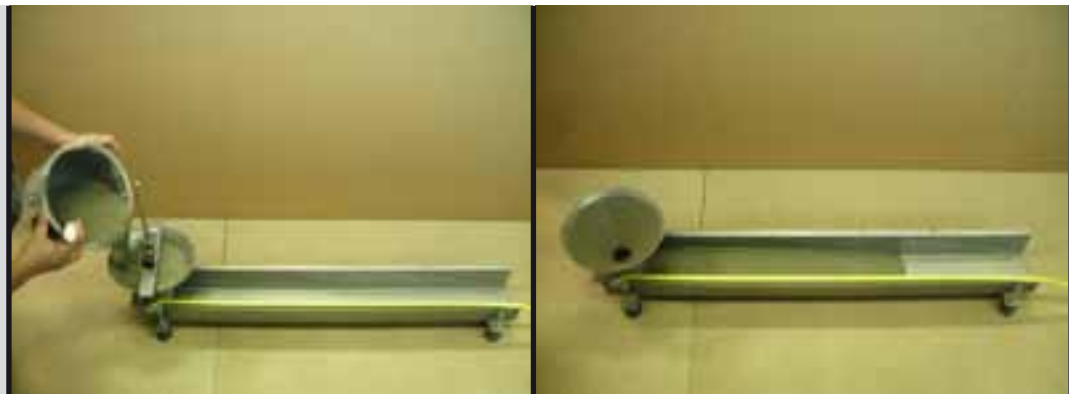
photo 3 - photo 4 Equipment used to carry out a flow test
