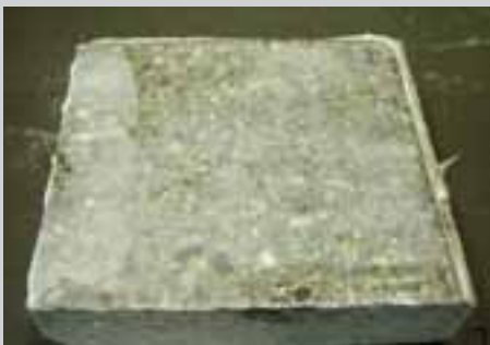
Appearance just after spreading Mapecrete Creme Protection
