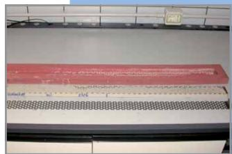
However, the method described above only allows dimensional variations of the samples to be measured after hardening, and does not allow the behaviour of the product during the plastic phase to be monitored. It is during this phase that the product is subject to higher transformation of its mechanical properties, passing from a fluid state to a solid state.
