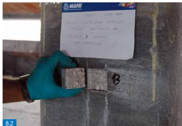
Figure 8.2 - Cohesive failure of the substrate
