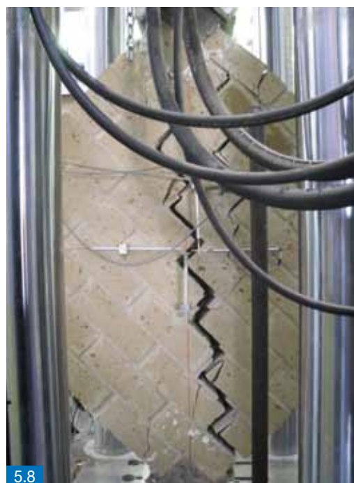
Figure 5.8 - The behaviour of a masonry panel without strengthening
