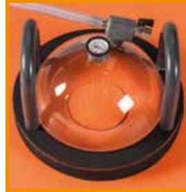
IV Vacuum Bell Test – joints/patch
