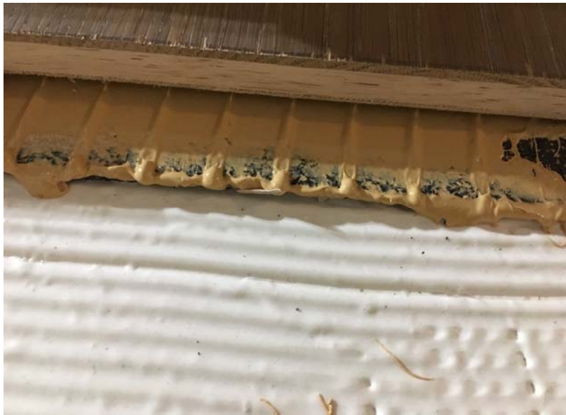
Figure 4: Sample showing flooring, underlay and both Mapei adhesives.
