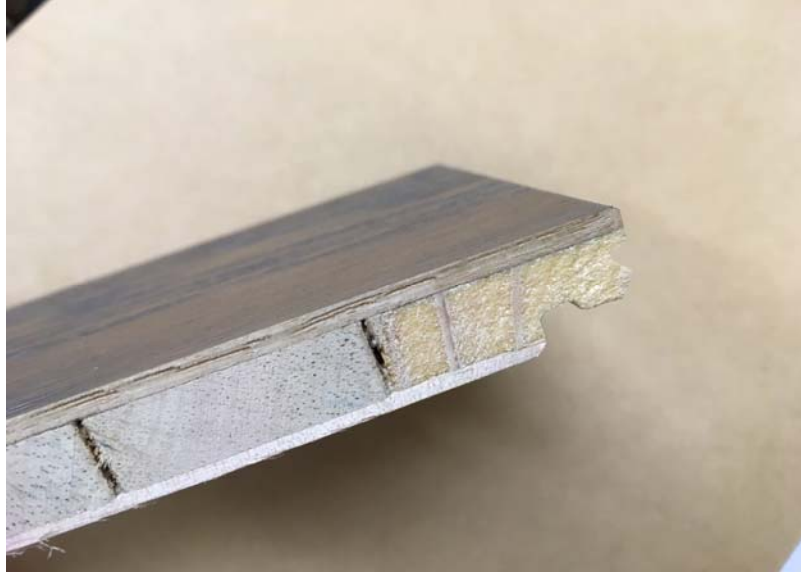
Figure 1: Section view of Godfrey Hirst-14.5 mm Oak timber laminate flooring
