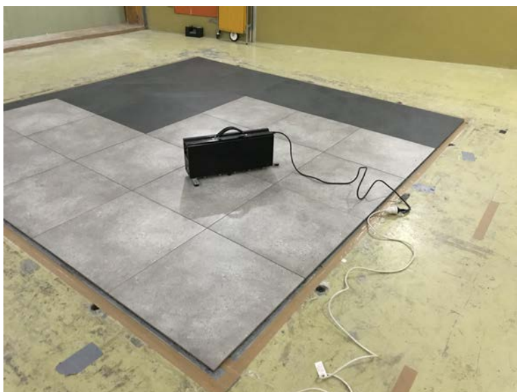
Figure 1.6: Impact tapping machine on sample
