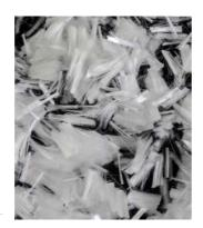
DOSAGE 600 g/m<sup>3</sup> of concrete or mortar
