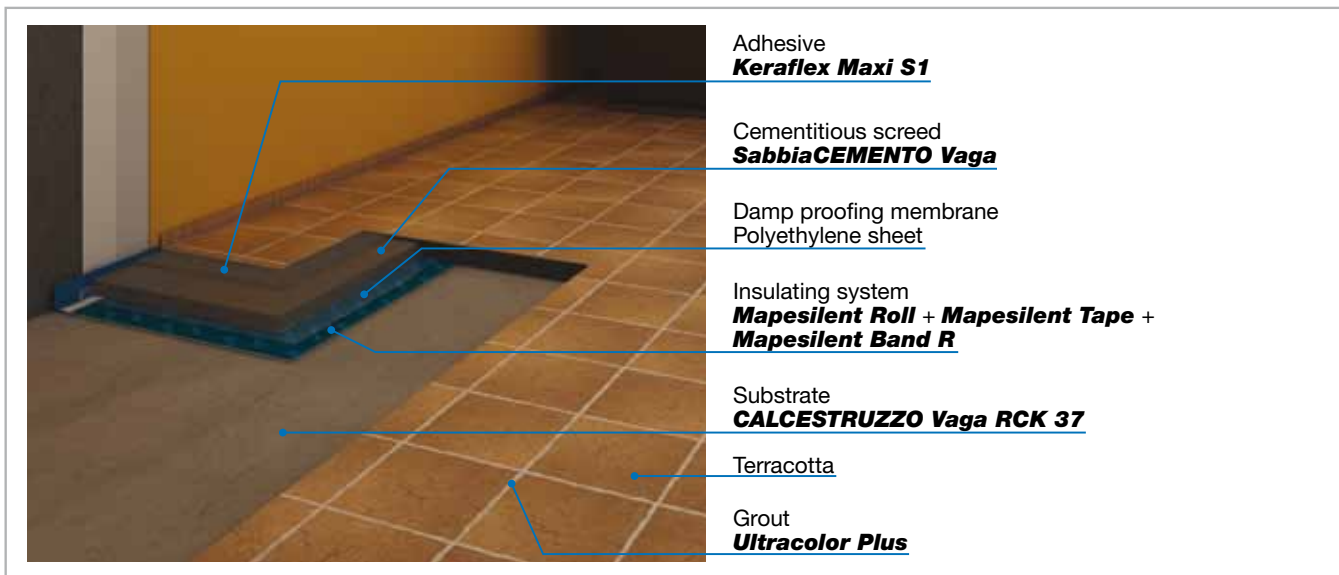
Fig. 4.3.2 - Floating screed soundproofed with MAPESILENT SYSTEM
