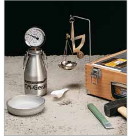
Fig. 3.5 - The most reliable instrument to measure residual moisture in a screed is a carbide hygrometer
