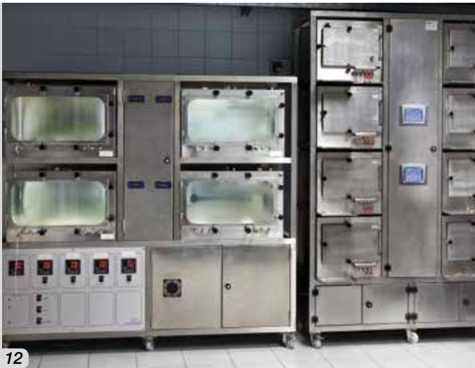
Fig. 12 - Environmental simulation chambers available at the Mapei R&D laboratory Figs. 13_14 - Test to measure VOC emissions
