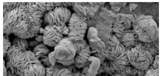
Fig. 8 - Tile joint with efflorescence viewed through an electron microscope
