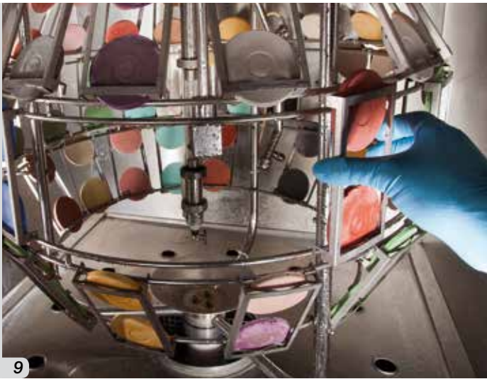
Fig. 9 - Accelerated ageing test using a weatherometer Figs. 10_11 - Verifying colour with a spectrophotometer
