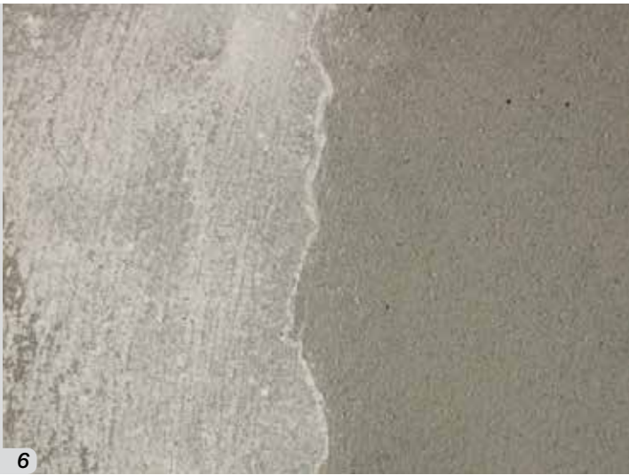
Fig. 6 - The surface of cementitious grout with efflorescence
