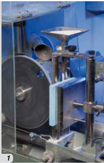
Figs. 1_2 - Test to measure abrasion resistance Fig. 3 - Verifying the stability of a sample of cementitious grout
